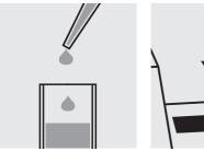
Pipette the sample into a 10 mm guartz photometer cell cell.
