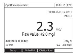
In addition to the measured value, an evaluation number for the measurement quality (MQ) is shown on the display.
